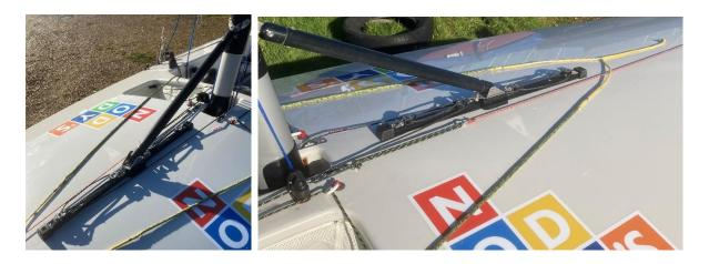
Strut/ Ram system with track on the deck. The jib cunningham line and cleat is also in veiw.
