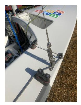
Jib bar system showing simple and calibrated adjustment. Shroud adjustment by pin system, reaching cleat on raise pad in chosen position.
