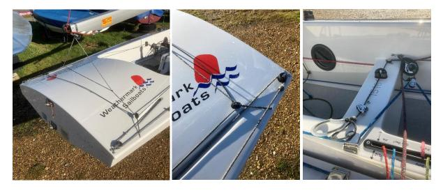
Aft Mainsheet bridal system showing lead to control on thwart.
