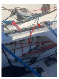
Spinnaker halyard pump cleat show extra cleat to prevent unwanted launching.
